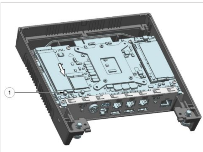
Figure 12-10: Removing the SSD
