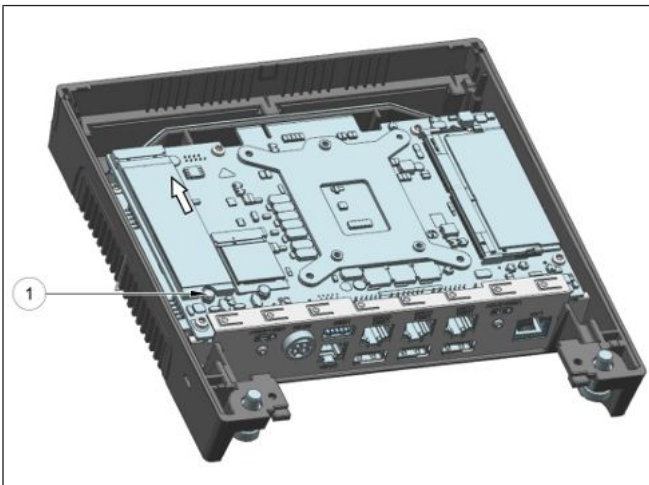
Figure 12-11: Inserting a new SSD
