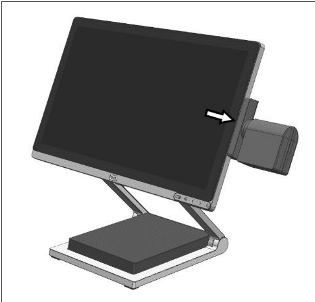
Figure 15-38: Snapping back the BCR top cover
